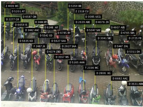
Figure 1.2 Implementation of OCR Algorithm in Small Parking Areas
